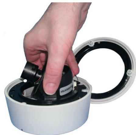
To rotate gimbal in base, hold by hinges & turn
