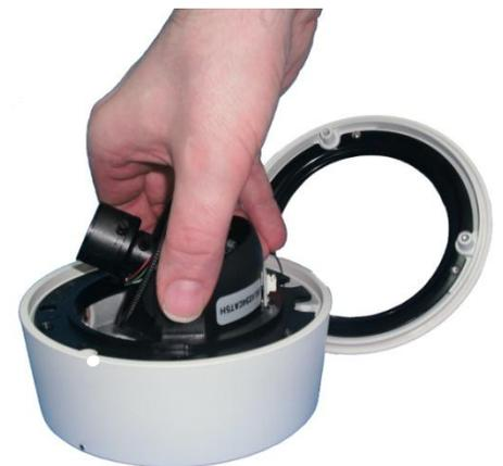
To rotate gimbal in base, hold by hinges & turn
