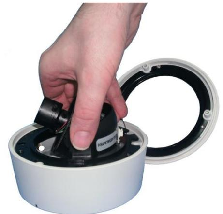
To rotate gimbal in base, hold by hinges & turn
